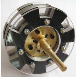
Fig. 8. View of a rotor comprising a shaft, fixing flanges, a magnet enclosure, rotor sections and stratified laminations and side perspex panels with brass bolts to tighten the rotor body
